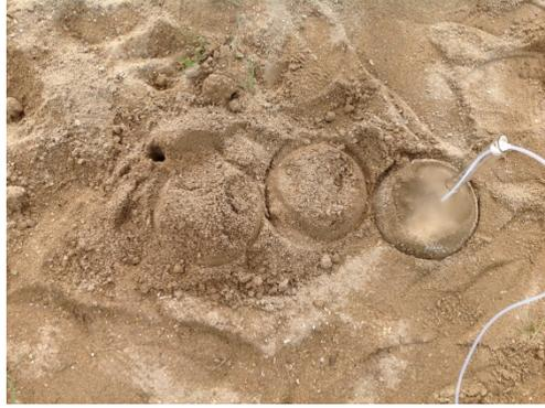
**Figure 7. The Sampling Funnel, displaced by 40 cm from the Burial Site for the Oil Sample (First Ring)**
