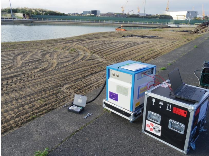
**Figure 2. PTR-MS (Blue Box) Set-up for the Oil Detection Trials on CEDRE's Artificial Beach.**
